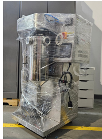
Our new spray dryer makes it easier to gently harvest fermented microbial cells for better downstream application analysis
